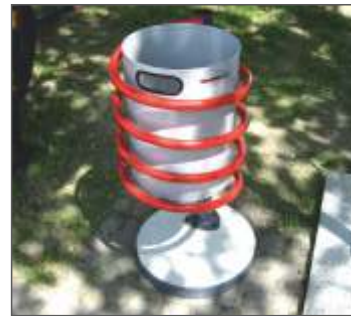
TYPE 2602 - Trash can round Stand: steel Basket: steel Volume: 35 L Dim.(LxBxH): 515x400x850 mm
