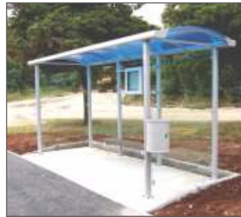
TYPE 1310 - Bus stop shelter Construction: aluminum Back side: glass Sides: glass Roof: polycarbonate or composite al Dim.(LxBxH): 5000x1750x2530 mm
