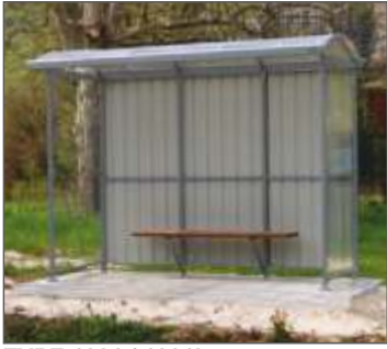
TYPE 1001 / 1001I Bus stop shelter Construction: inox or steel Back side: glass or sheet metal Sides: glass or polycarbonate Roof: polycarbonate or composite al Dim.(LxBxH): 3100x1540x2450 mm
