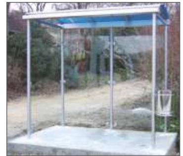
TYPE 1260 - Bus stop shelter Construction: inox Back side: glass Sides: glass Roof: polycarbonate or composite al Dim.(LxBxH): 2500x1640x2500 mm
