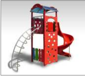
TYPE 8510 - Spiral slide with tower Construction: aluminum and steel Mask: HDPE Slide: polyester Dim.(LxBxH): 6275x2000x4000mm
