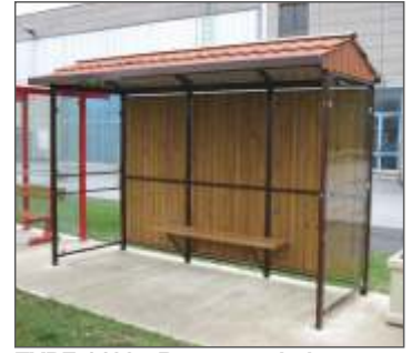
TYPE 1400 - Bus stop shelter Construction: steel Back side: wood Sides: glass Roof: profiled sheet Dim.(LxBxH): 3690x1560x2570 mm
