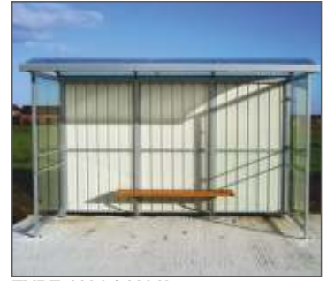
TYPE 1101 / 1101I Bus stop shelter Construction: inox or steel Back side: trapezoidal sheet Sides: glass Roof: polycarbonate or composite al Dim.(LxBxH): 3690x1540x2450 mm
