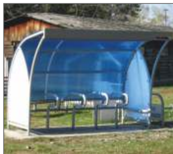
TYPE 1807 - Shelter for bikes Construction: steel Cover: polycarbonate or composite al. panel Dim.(LxBxH): 3060x2050x2200mm Places for bicycles: 5
