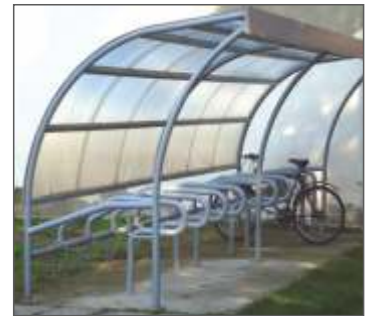
TYPE 1800 - Shelter for bikes Construction: steel Cover: polycarbonate or composite al. panel Dim.(LxBxH): 6060x2050x2200mm Places for bicycles: 10
