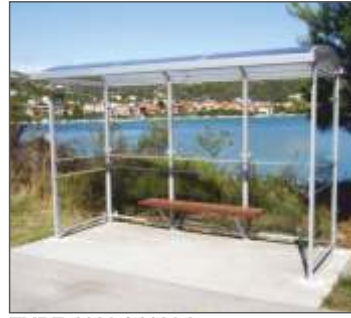
TYPE 1100 / 1100 I Bus stop shelter Construction: inox or steel Back side: glass Sides: glass Roof: polycarbonate or composite al Dim.(LxBxH): 3690x1540x2450 mm
